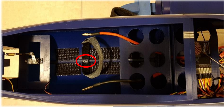
Possible battery lock system with rigid adhesive velcro and screw fastened strap.
