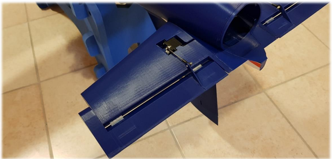
Glue the tail to the fuselage and install the elevator
