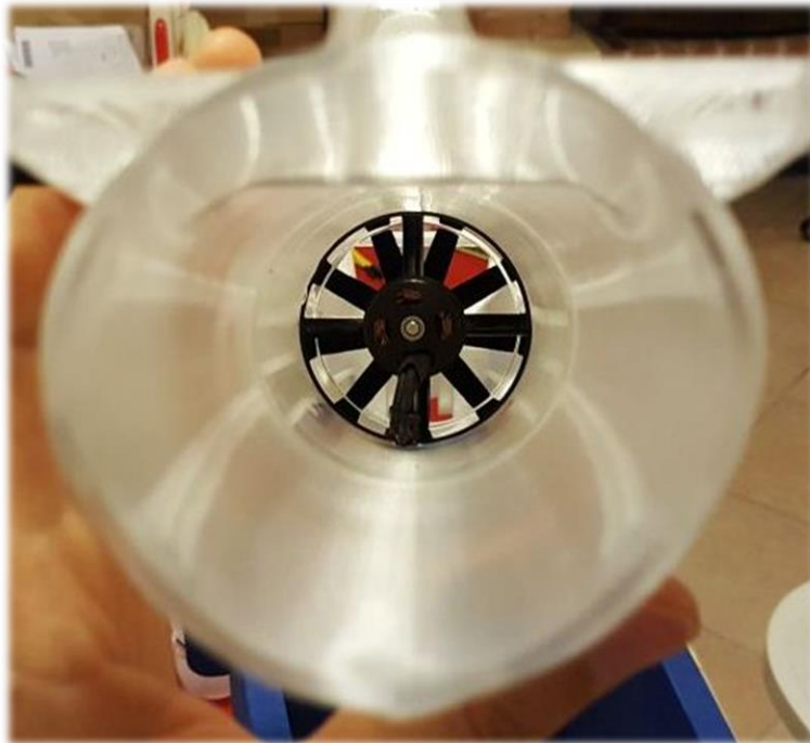
Details venturi rear final section
